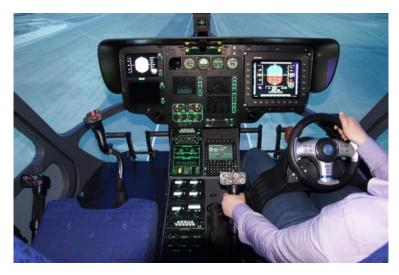
Figure 9. Steering wheel control for a personal aerial vehicle [44].
