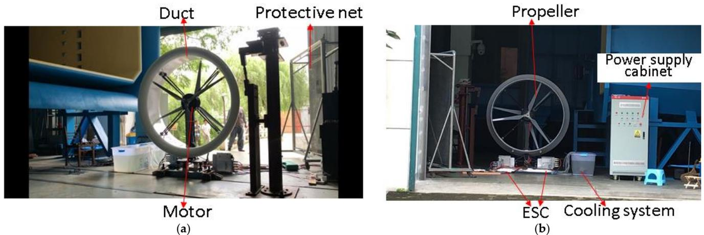
Figure 8. Lift and power measurement test bench: (a) duct inlet; (b) duct outlet.
