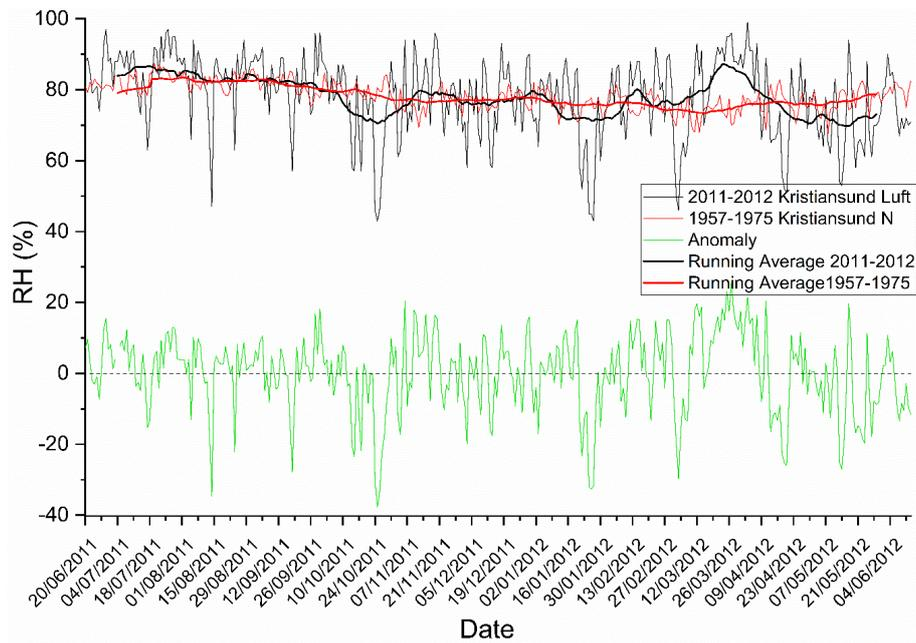
**Figure 2S:** Upper part - Daily outdoor relative humidity (%) registered at the Kristiansund Airport Meteorological station between 20/06/2011 and 13/06/2012 (Thin black line and thick black line for the running average) and at the Kristiansund N Meteorological station for the normal period 1957-1975 (Thin red line and thick red line for the running average). Bottom Part – RH Anomaly (%) (Green thin line) between the data recorded in 2011-2012 and the reference period (1957-1975).
