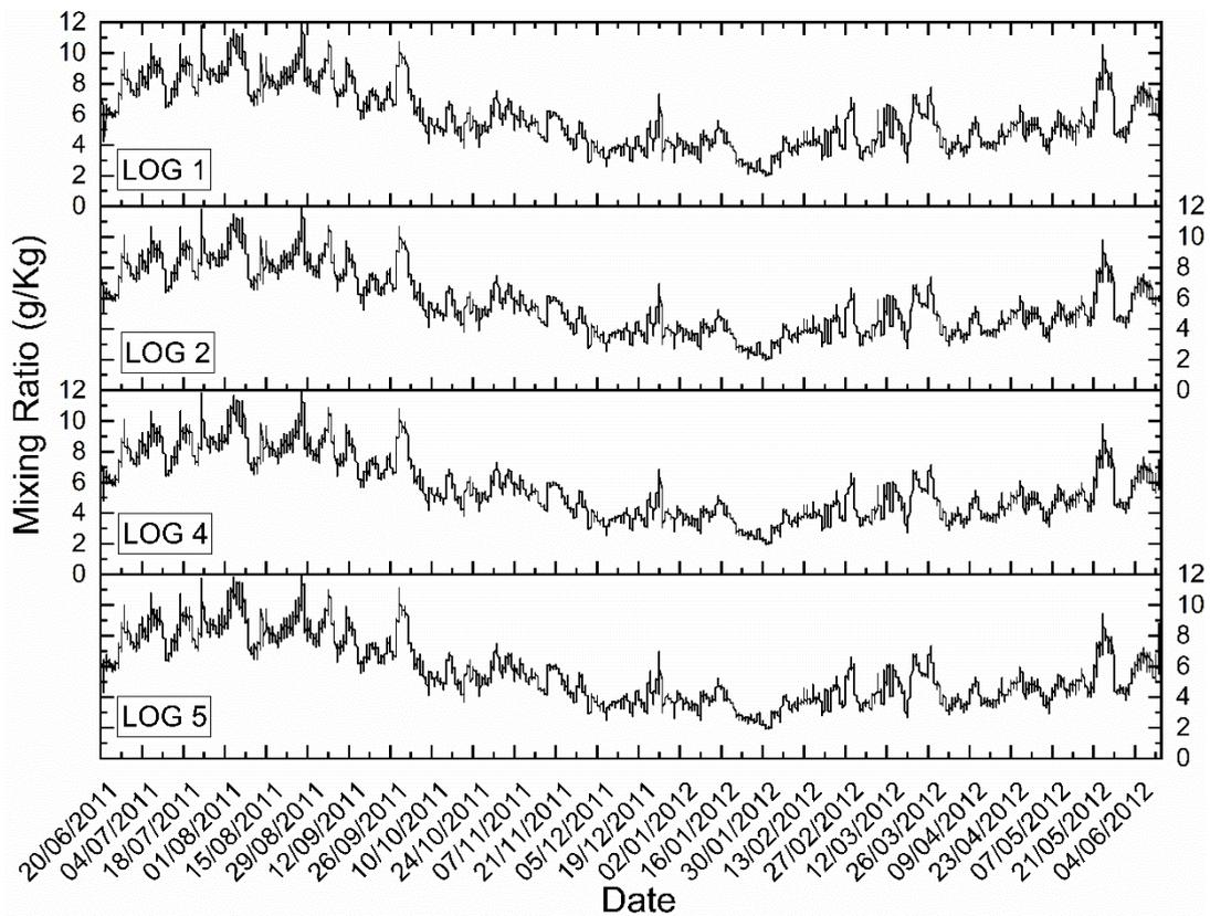
**Figure 5S:** Indoor mixing Ratio values obtained for the 4 data logger between 20/6/2011 and 13/6/2012 every 2 hours
