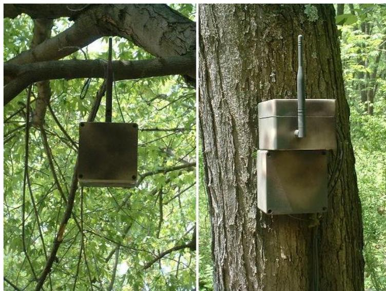
Tolle *et al.* [17] deployed 33 WSN nodes to monitor a redwood tree during 44 days. The deployment used battery-powered Mica2Dot nodes and the analysis shows a 49% data yield, considering that some
