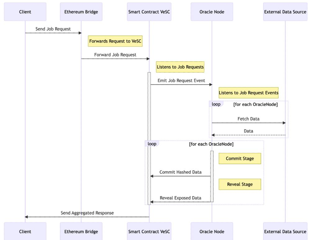
Figure 2. API Job lifecycle sequence diagram.
