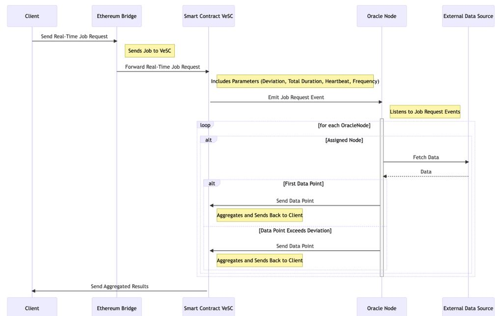
Figure 3. Real-time Job lifecycle sequence diagram.
