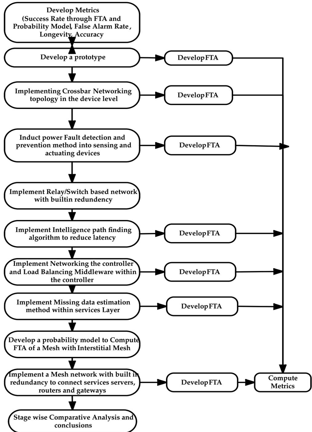
Figure 1. Overall computational strategy to enhance fault tolerance in the gateway layer.
