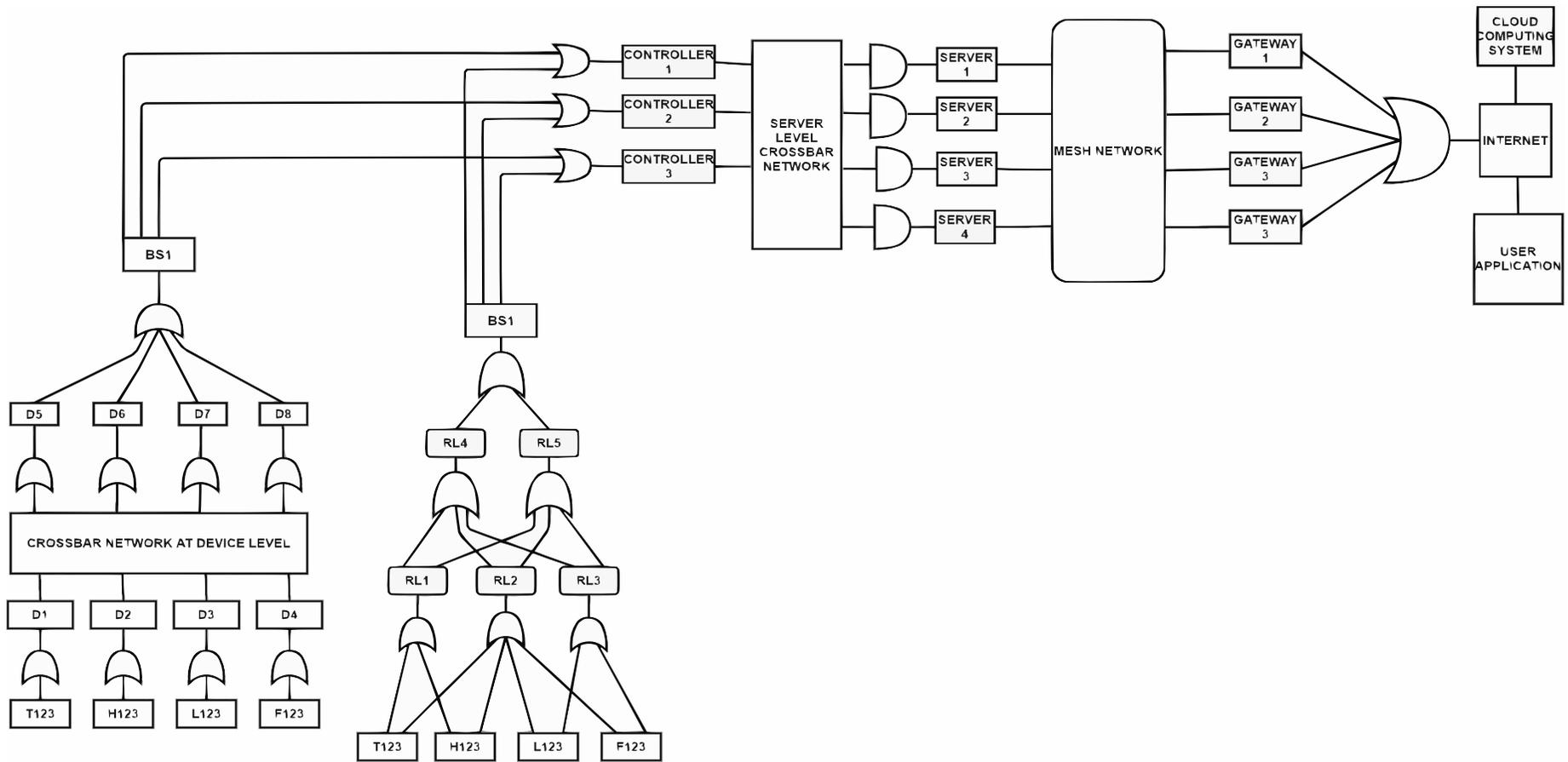
Figure 8. Revised FTA diagram.
