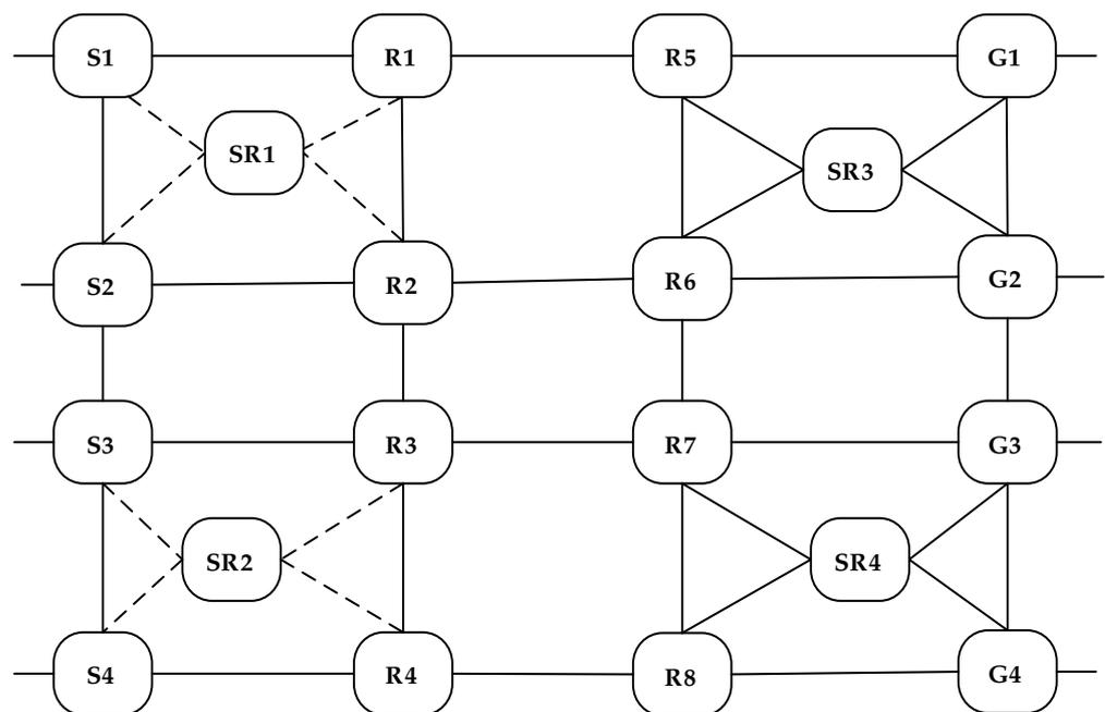
**Figure 3.** Mesh network connecting service’s servers to the gateway. S1, S2, S3, S4 = servers. SR1, SR2, SR3, SR4 = spare routers. G1, G2, G3, G4 = gateways. R1–R8 = routers.
