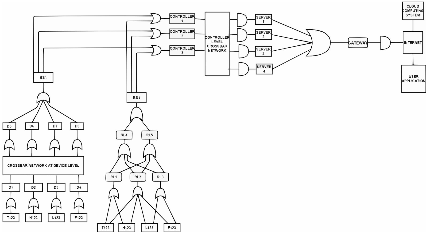
Figure 6. FTA diagram for the example IoT network.
