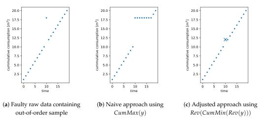
Figure 4. Approach for removing out-of-order samples that violate the monotonic constraint.
