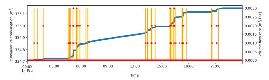
**Figure 6.** From the series of measured values, V(t)-derived times of human activity events (orange lines) in the analogous time slot to Figure 5.
