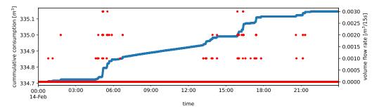
**Figure 5.** A sample extract of the series of measured values after pre-processing V(t) over one day (blue), as well as the derived volume flow rates series q(t) (red). (Household: WM-A-08; Day: 2022-02-14).
