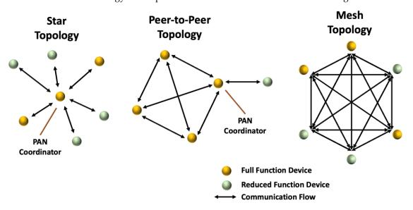
Figure 8. Illustration of various network topology types [45].
