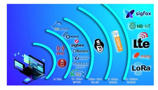
Figure 4. Illustration of existing technologies for wireless networking regarding connectivity range.
