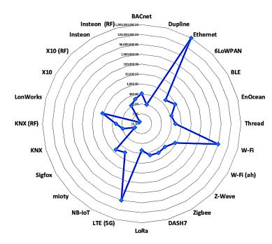
Figure 6. Data rates of home automation technologies (Kbps).
