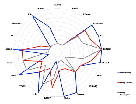
**Figure 12.** Graphical comparison of existing networking technologies regarding energy/cost, from minimum to maximum gain.
