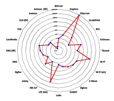
Figure 7. Data rates to packet sizes ratio (minimum to maximum).
