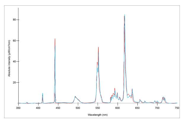
Figure S1: Comparison of the spectral output of a new fluorescent lamp (blue line) with one approximately six months old (red line).
