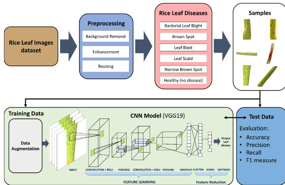
**Figure 1.** Proposed deep convolutional neural networks (CNN) transfer learning-based approach for leaf disease classification.
