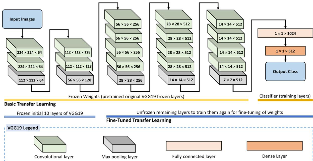
**Figure 4.** Fine-tuned transfer learning for the VGG19 model for rice leaf disease identification.
