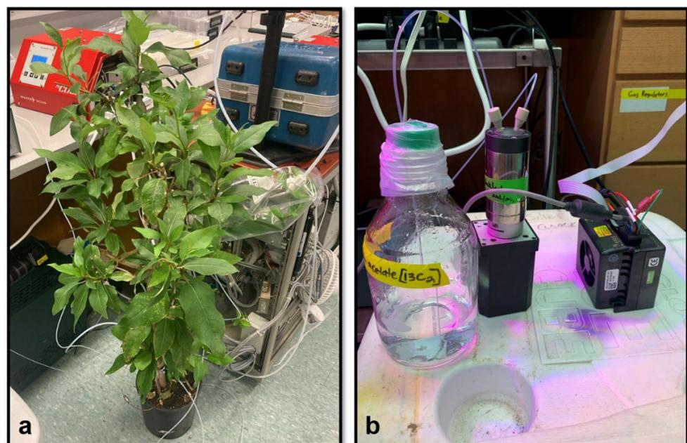
**Figure 2.** Images showing the (a) DXSI experimental set-up in the laboratory and (b) M6 pump and 500 mL solution reservoir.
