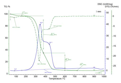
**Figure 4.** Results of simultaneous thermal analysis in the air atmosphere on the example of BWW with a nine-year storage period.
