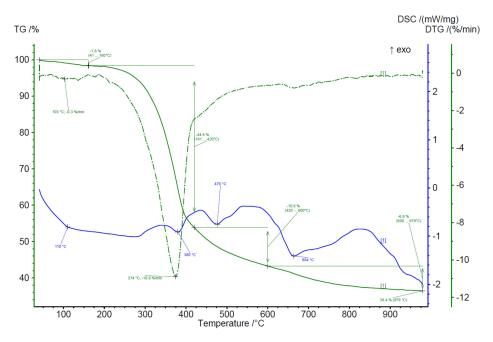
**Figure 7.** Results of simultaneous thermal analysis in the air atmosphere on the example of BWW with an 82-year storage period.
