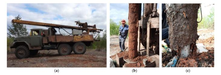
**Figure 2.** Sampling process: (**a**) URB-2A drilling rig; (**b**) general view of the drilled core; (**c**) BWW condition and structure.
