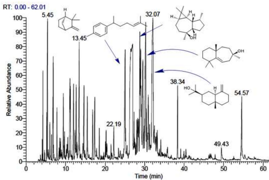
**Figure S1.** Chromatogram and structures of the main components of the essential oils of *A. monosperma*.
