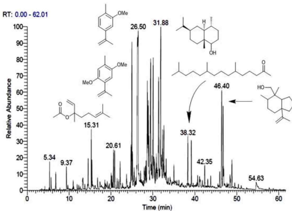
**Figure S2.** Chromatogram and structures of the main components of the essential oils of *L. crithmoides*.
