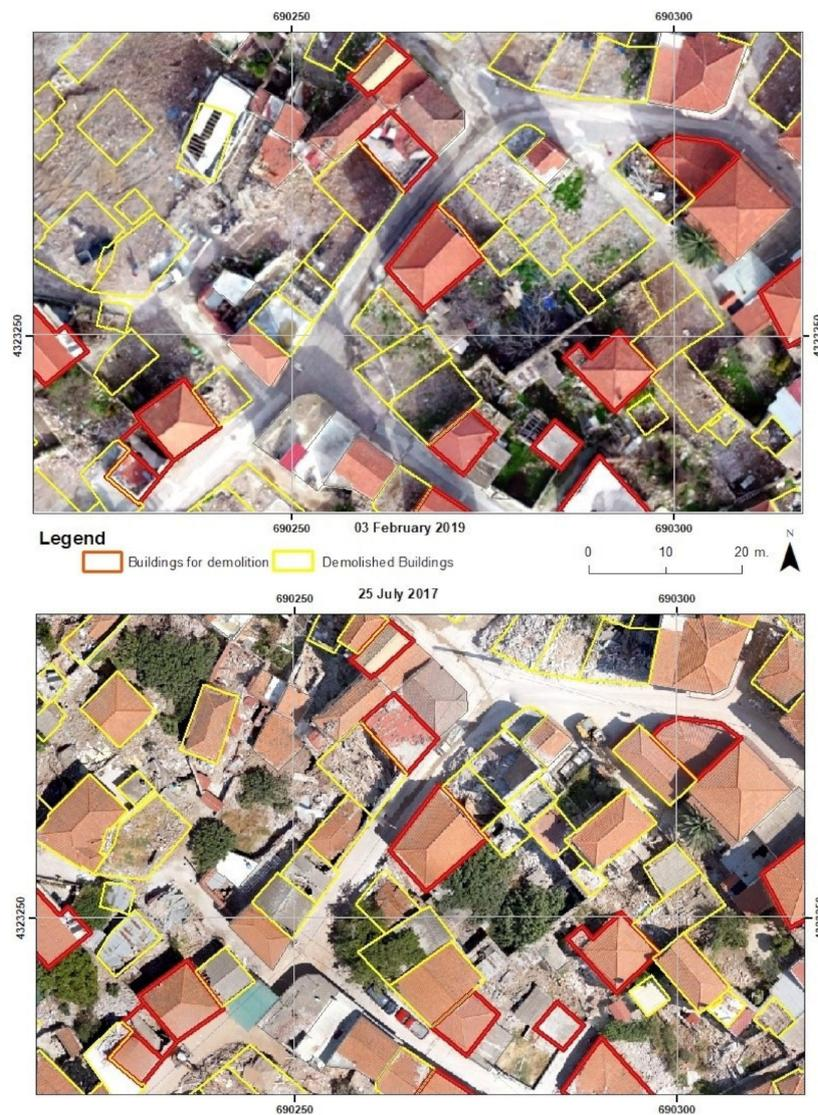
**Figure 6.** The top orthophoto map of 3rd February 2019 derived from UAS 4K-video footage presents the demolished buildings mapped by photo interpretation and fieldwork. The bottom orthophoto map of 25th July 2017, derived by UAS high resolution images, presents the buildings which have been approved for demolition by the Greek-EPO.
