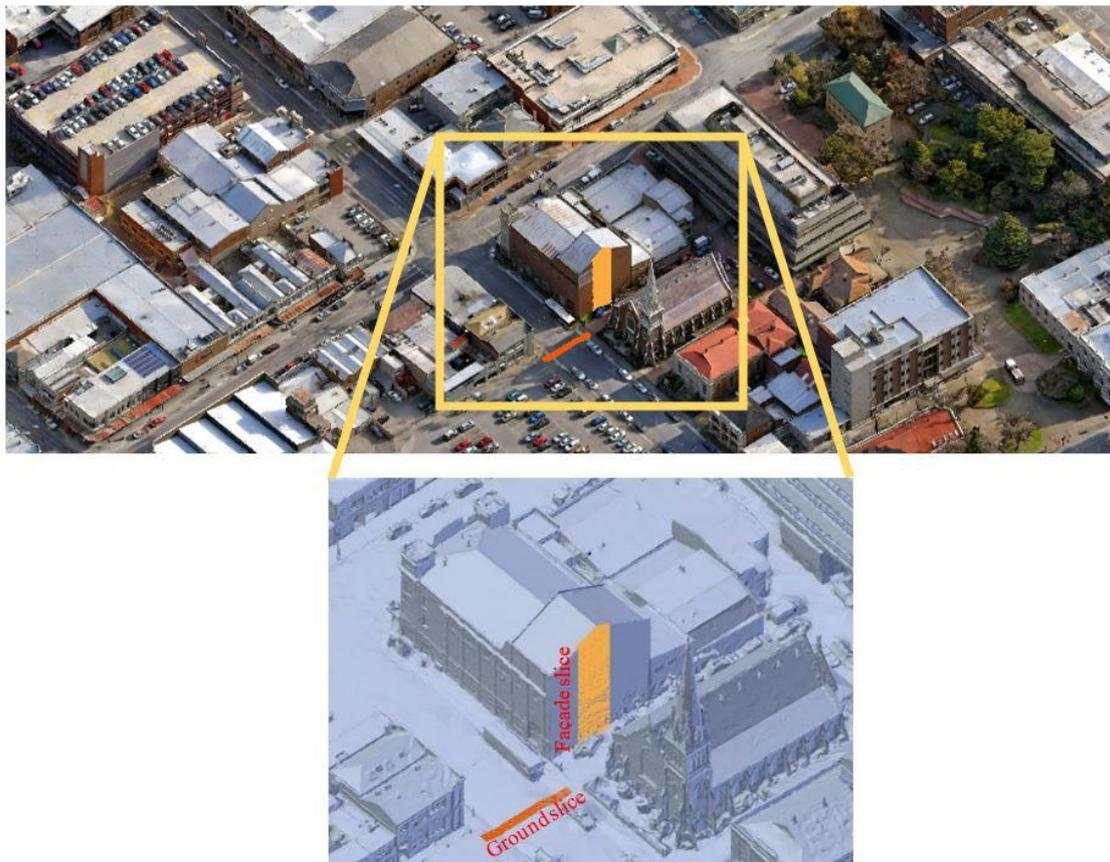
**Figure 18.** Two selected slices, on the ground (orange) and on a building facade (yellow), to check the achieved LiDAR point density.
