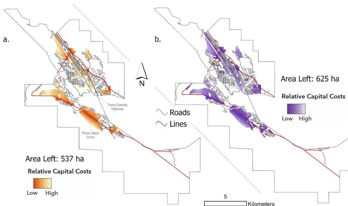
**Figure 6.** Relative capital cost of connecting those resources to existing roads and lines after constraint applied for (a) solar and (b) wind opportunities. Constraints include technically recoverable resources and those semi-permissive lands under legally accessible resources.
