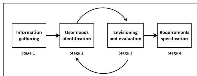
**Figure 4.** General process for users' requirements analysis. Source: Adapted from [14].
