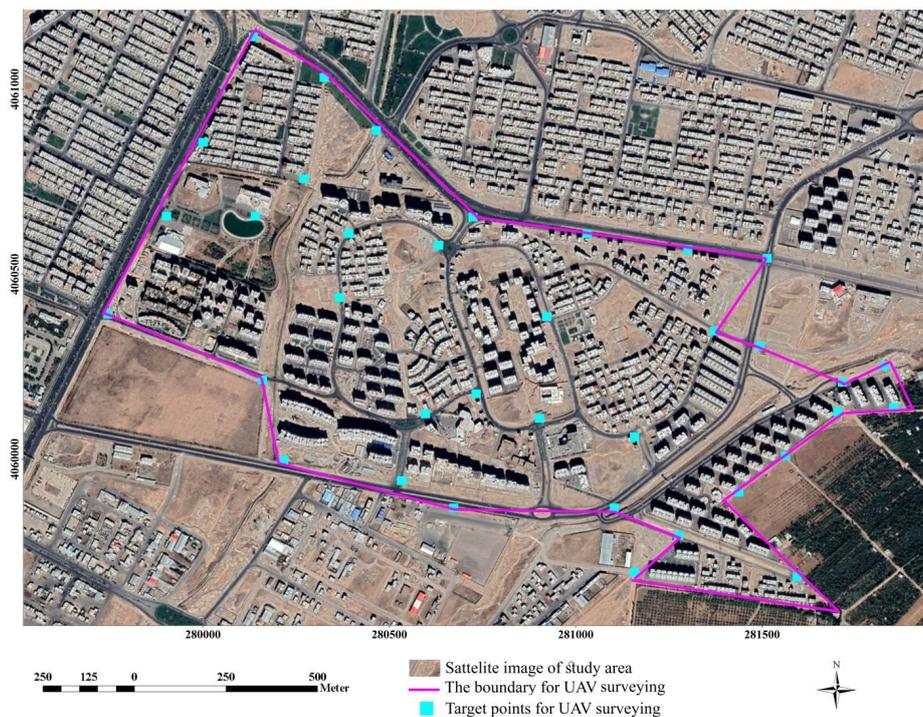
**Figure 3.** The distribution of target points for unmanned aerial vehicle (UAV) surveying in the study area (the blue points show the targets and the pink polygon shows the area for UAV surveying).
