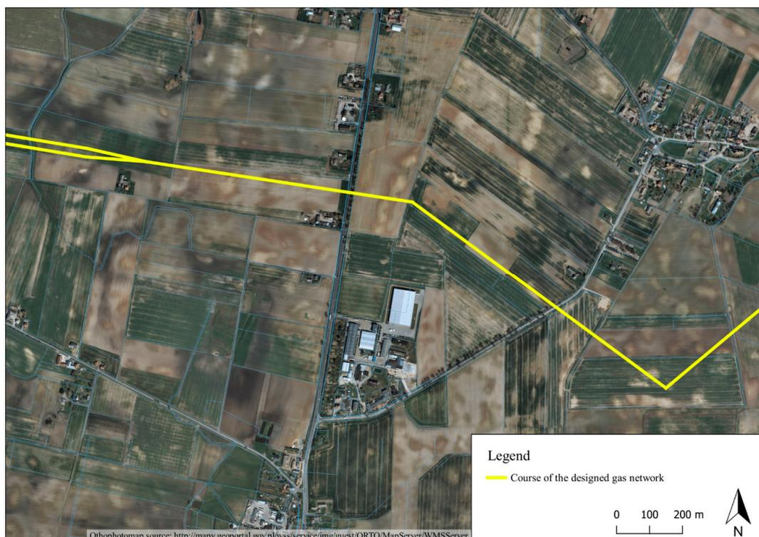
Figure 4. Marking of the gas network. Source: Own study based on [16].
