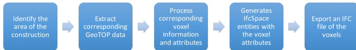
Figure 10. Workflow of this solution.
