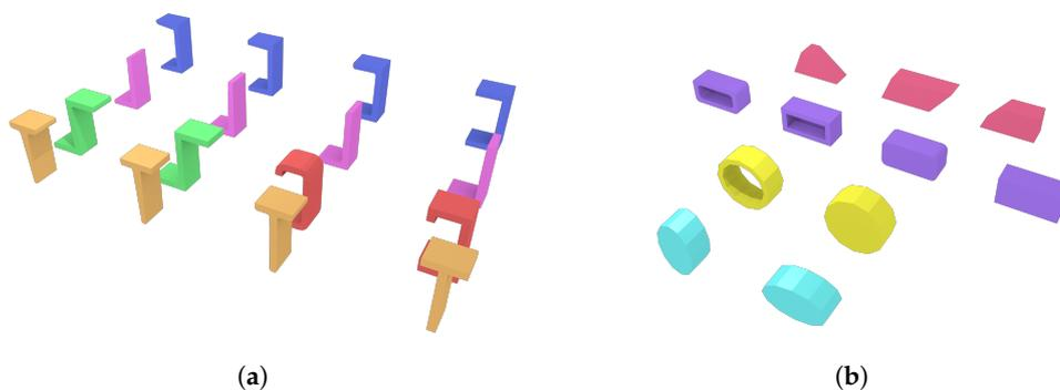
**Figure 2.** IFC defines various types of parametric curved profiles such as (a) those based on the characters U, L, Z, C and T and (b) those based on trapezia, (rounded) rectangles, circles with/without holes and ellipses. Note the various types of tapered and curved parts of the profiles. These are most commonly used in extrusions such as those shown here.
