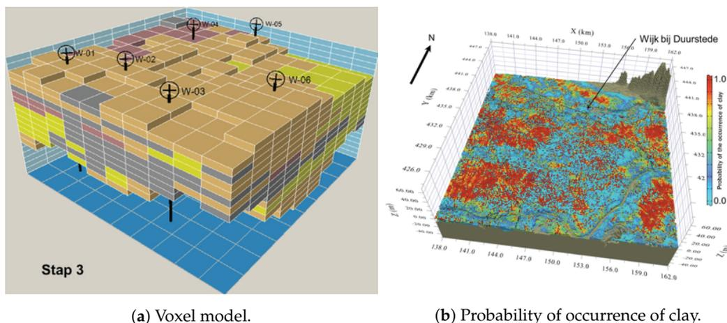
**Figure 9.** GeoTOP data is encoded based on a voxel model with a resolution of  $100 \times 100 \times 0.5$  m. Each voxel in the model contains information on the lithostratigraphy and lithological classes, including the probability of occurrence for each lithological class (the values are based on interpolations of data from boreholes).
