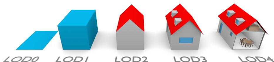
**Figure 1.** A building represented in LOD0 to LOD4 (image from Biljecki et al. [12]).
