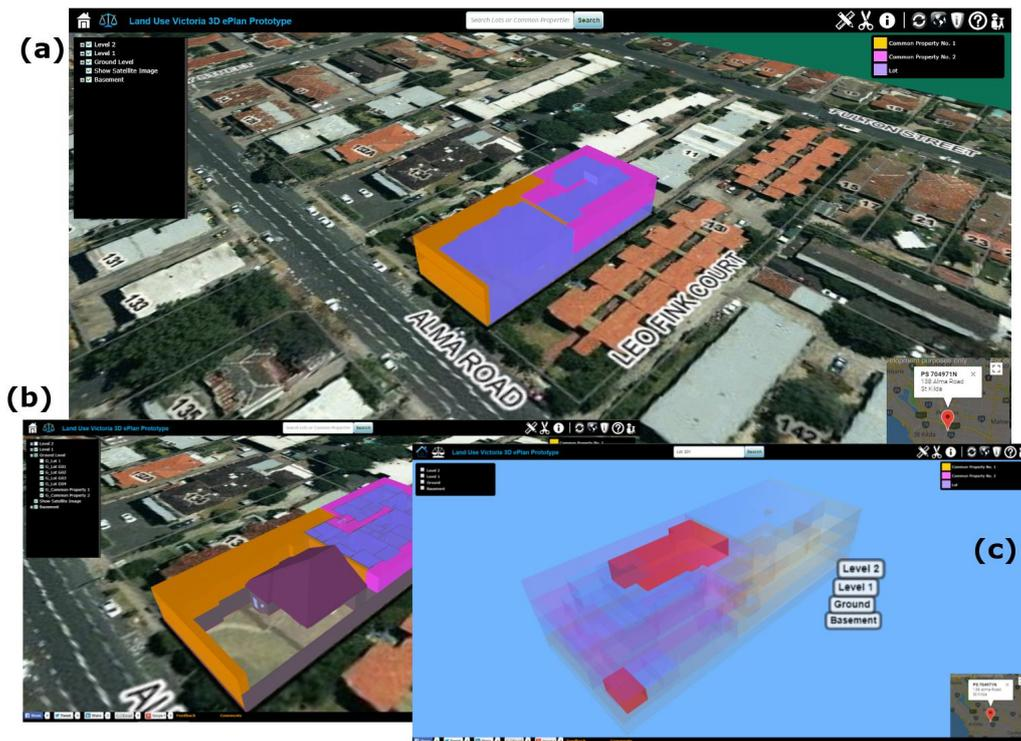
Figure 4. (a) A snapshot of the prototype ([www.spear.land.vic.gov.au/spear/pages/eplan/3d-digital-cadastral/3dprototype/prototype.html](http://www.spear.land.vic.gov.au/spear/pages/eplan/3d-digital-cadastral/3dprototype/prototype.html)). (b) A combined visualization of the building (physical and legal view). (c) Search of a lot within the building displaying an apartment unit and its car park.
