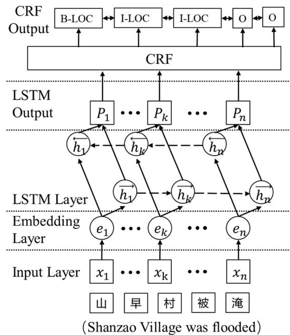
**Figure 2.** Flowchart of the Bi-LSTM-CRF algorithm.
