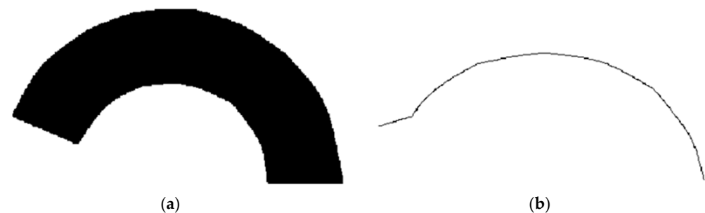
Figure 7. Projection thinning, from a binary image to a 2D topological map: (a) binary image; (b) 2D topological map.
