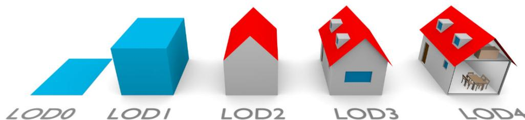
**Figure 1.** The five LODs of buildings in CityGML (image from [17]).
