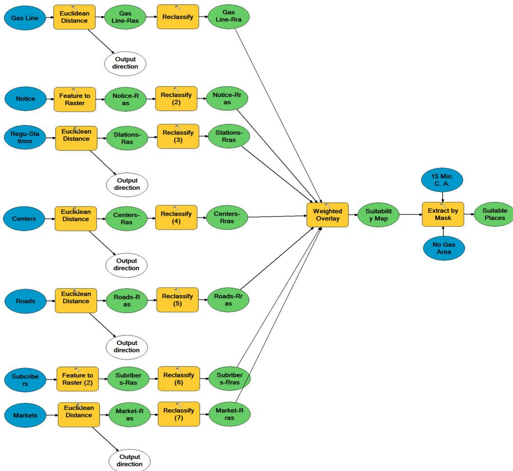
Figure 5. New natural gas emergency response team center location analysis model.
