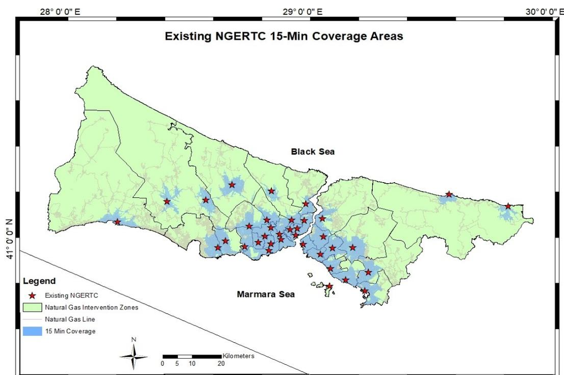
**Figure 6.** Natural gas emergency response team center 15 min coverage areas and natural gas intervention zones.
