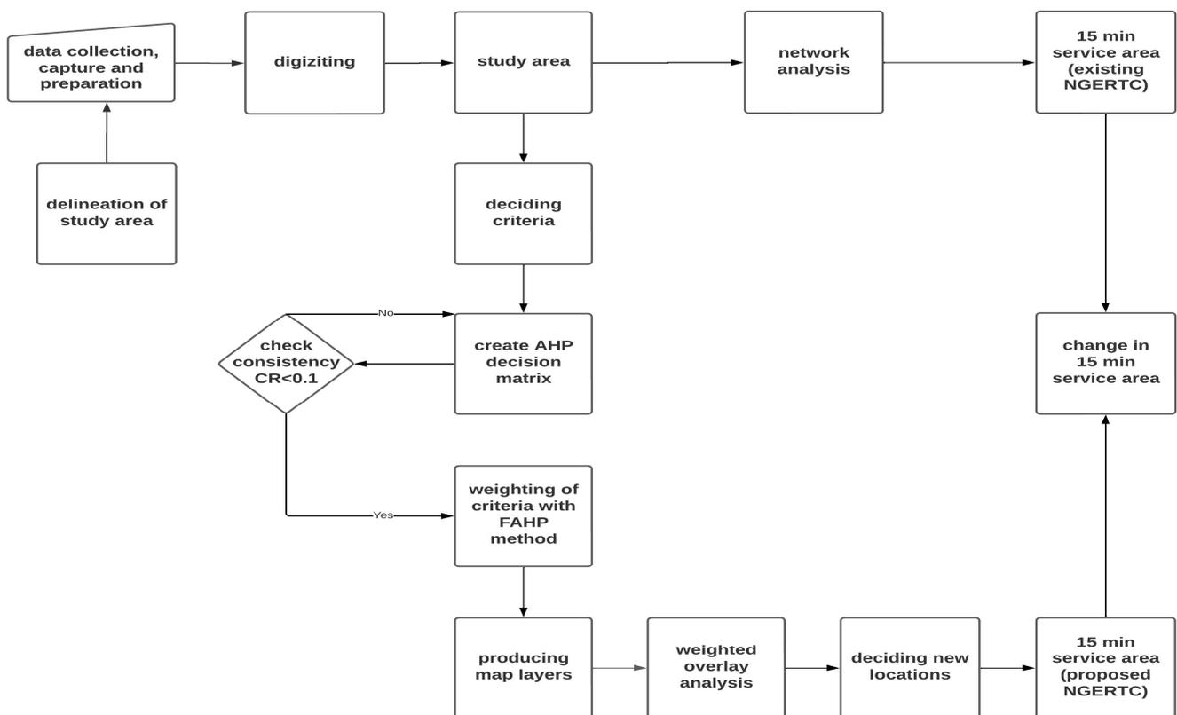
Figure 4. The workflow of site selection study of natural gas emergency response team centers.
