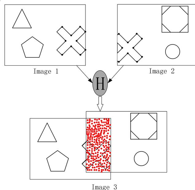
**Figure 1.** Image registration. The dark spots at the same position on image 1 and image 2 are a pair of known matching points. We can use them to calculate the homography matrix  $H$  and then use  $H$  to gain image 3.
