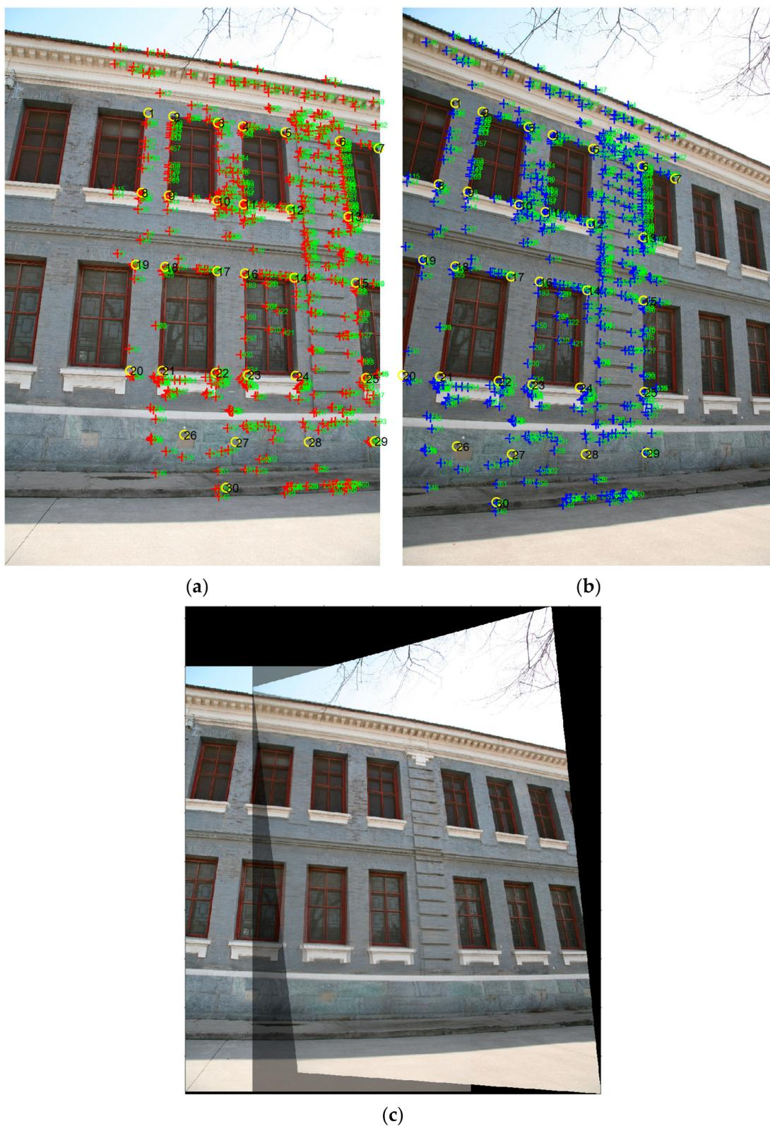
**Figure 5.** Primary data of the real scene (Robot Vision Group (ia.ac.cn)). (a) Left image. (b) Right image. (c) Registered image. The '+' and 'o' points with the same number on the left and right images represent a pair of matching points and a pair of control points, respectively.
