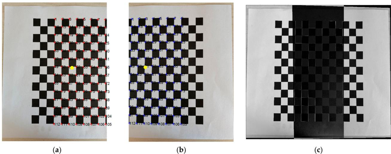
**Figure 3.** Primary data of the simulation scene. (a) Left image and the feature points. (b) Right image and the feature points. The symbols + with the same number in (a,b) are a pair of known matching points. The yellow dots are the center points of the overlapping region of the left and right images. (c) Registered image.
