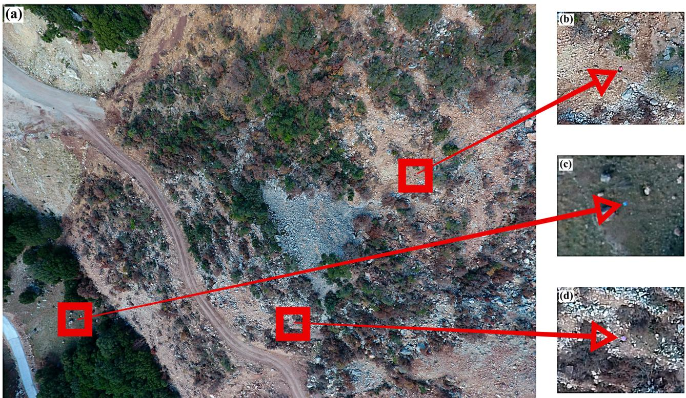
Figure 3. (a) UAV image acquired on 5 November 2017. The red squares define the area where GCPs are located. (b–d) GCP patterns as recognized in UAV imagery.
