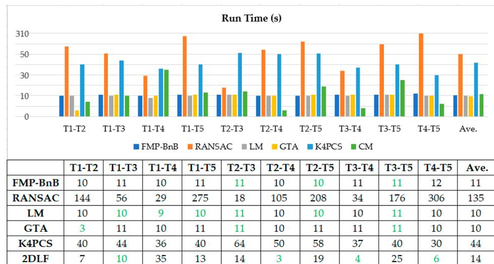
Figure 11. Run time to register point cloud pairs from dataset SR (the most time-efficient method for each pair is colored in green).
