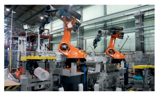
**Figure 1.** Box Encapsulation Plant (BEP) robot rig trial being carried out at National Nuclear Laboratory (NNL)'s rig hall in Workington, Cumbria, UK.
