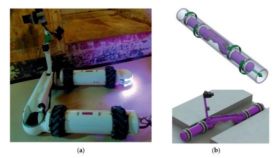
Figure 3. MIRRAX: (a) surveying an area; (b) omnidirectional capabilities.
