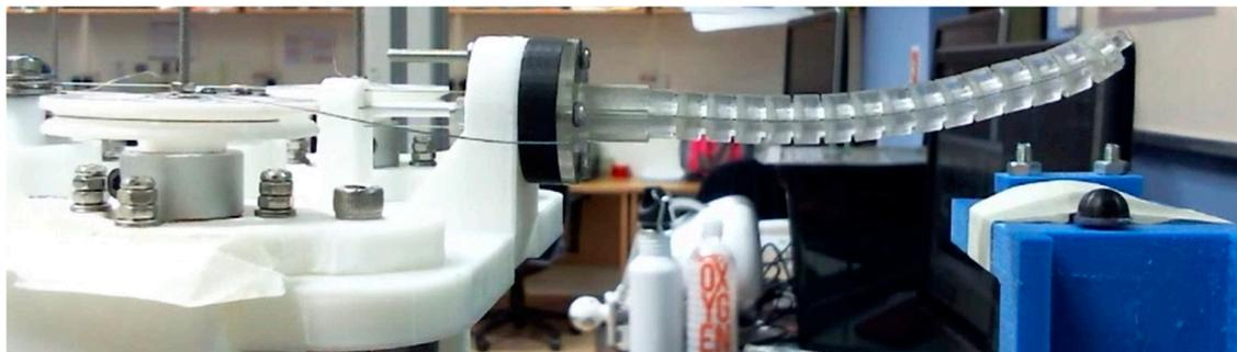
Figure 1. The wire-driven flexible manipulator (WDM) with direct drive mechanisms [25].
