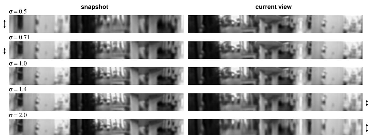
**Figure 4.** Scale-plane stack obtained from the image pairs in Figure 3. The scale factor  $\sigma$  is shown for each scale plane. Dark values indicate good matches between columns.
