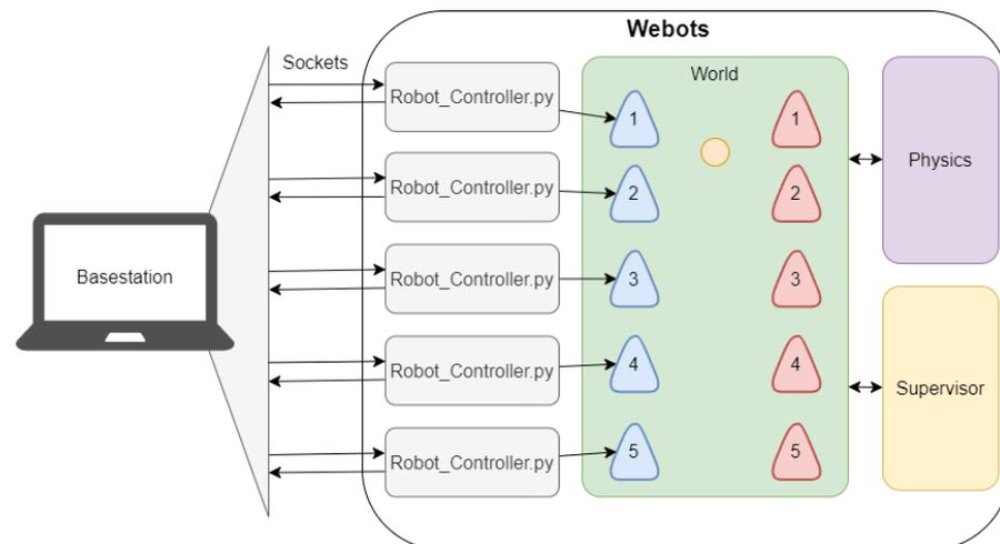
**Figure 24.** The architecture of the developed Webots simulation environment.
