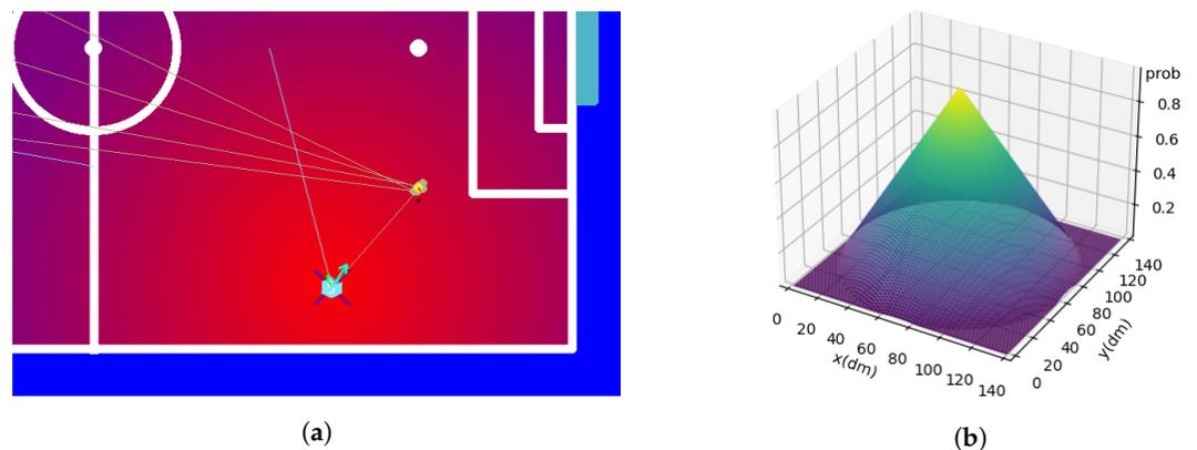
**Figure 13.** Representation of a base map based on the distance to the robot: (a) Two-dimensional base station representation. (b) Three-dimensional representation.
