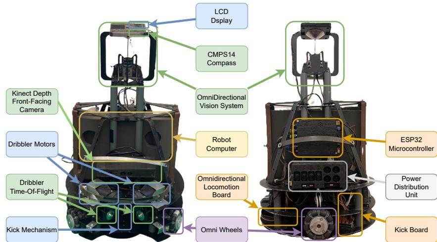
Figure 3. Robot photo with the main elements highlighted (front and back views).
