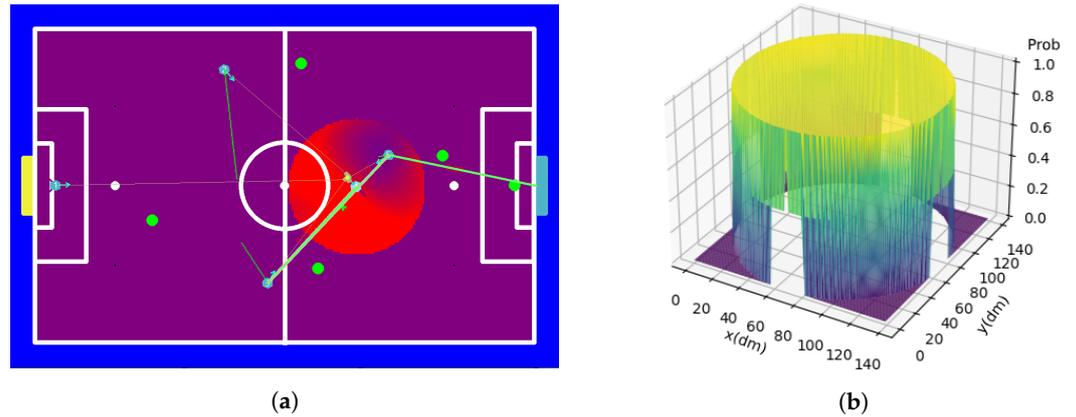
Figure 20. Three-meter radius rule map: (a) Field situation. (b) Three-dimensional matrix representation.
