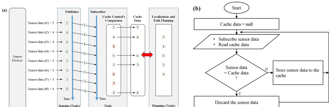
Figure 3. (a) Cache control works in the CEDDP; and (b) cache control flowchart.
