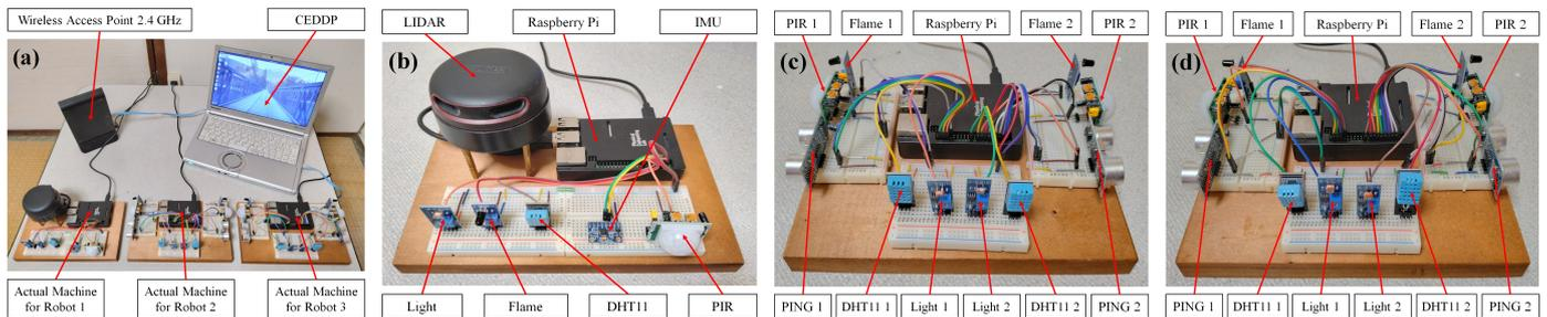
Figure 5. (a) Experimental setup on the actual machine; (b) sensor devices connected to the actual machine 1; (c) sensor devices connected to the actual machine 2; and (d) sensor devices connected to the actual machine 3.
