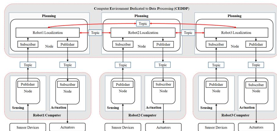
Figure 1. Aggregated robot processing architecture.
