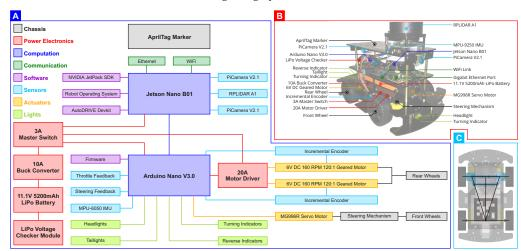
**Figure 2.** Native vehicle (Nigel) of the AutoDRIVE Ecosystem: (**A**) high-level vehicle architecture; (**B**) various components and sub-systems of the vehicle; (**C**) open-source chassis of the vehicle adopting rear-wheel drive, Ackermann steered actuation mechanism.
