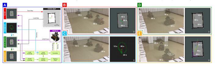
**Figure 5.** Autonomous parking: **(A)** high-level architecture of the autonomy algorithm; **(B–E)** respectively depict temporal analysis of simultaneous localization and mapping, odometry, localization, and navigation modules—(i) physical vehicle driving in real-world settings, (ii) visualization of software algorithm; note the additional boxes acting as unmapped obstacles in **(E)**. Video: <a href="https://youtu.be/oBqIZZA0wkc">https://youtu.be/oBqIZZA0wkc</a> (accessed on 9 May 2021).
