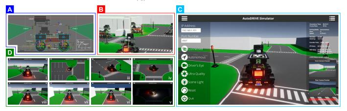
**Figure 4.** Native simulation platform of the AutoDRIVE Ecosystem: (**A**) simulation of vehicle dynamics, sensors and actuators; (**B**) simulation of infrastructure dynamics and interaction physics; (**C**) graphical user interface of the simulator; (**D**) simulator features—(i) Driver's Eye camera, (ii) Bird's Eye camera, (iii) God's Eye camera, (iv) scene light enabled, (v) scene light disabled, (vi) low-quality graphics, (vii) high-quality graphics, (viii) ultra-quality graphics.
