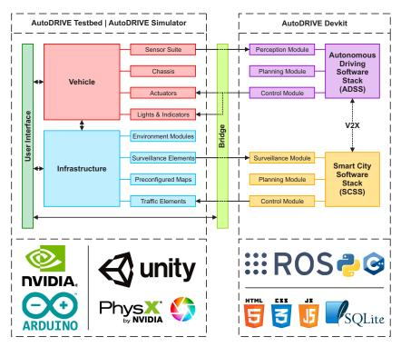
**Figure 1.** High -level overview of the AutoDRIVE Ecosystem, depicting the key modules and their interactions within the three platforms of the ecosystem, viz. AutoDRIVE Testbed, AutoDRIVE Simulator and AutoDRIVE Devkit.
