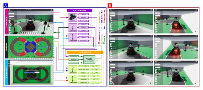
**Figure 8.** Smart city management: (**A**) high-level architecture of the autonomy algorithm; (**B**) snapshot instances from simulation—(i) vehicle observing left-curve sign, (ii) vehicle observing right-curve sign, (iii) vehicle crossing the intersection, (iv) vehicle stopping at red light, (v) vehicle stopping at yellow light, (vi) vehicle resuming on green light; the traffic lights are toggled manually. Video: https://youtu.be/fnxOpV1gFXo (accessed on 5 May 2021).
