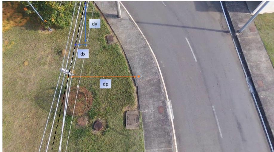
Figure 3. Extraction of errors using visual information.
