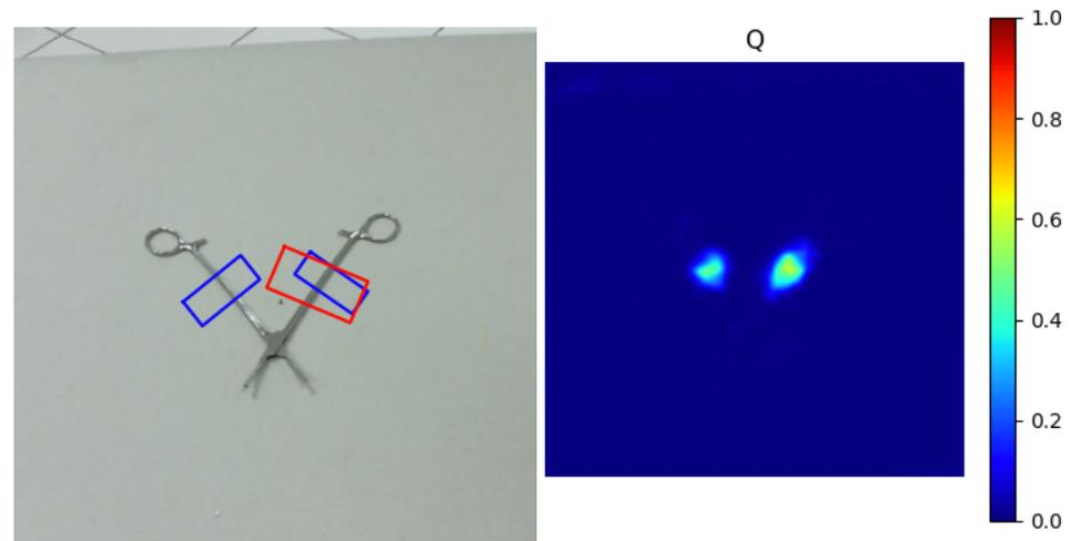
**Figure 4.** On the left, the real and ground-truth grasping rectangles; on the right, the  $q$  value of the image.
