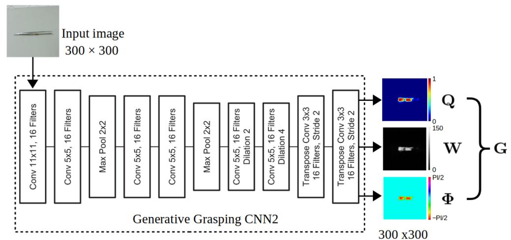
**Figure 2.** GG-CNN2 network architecture [2]. The GG-CNN2 directly generates a grasp pose  $G$  from grasp quality  $Q$ , grasp width  $W$ , and grasp angle  $\Phi$ .
