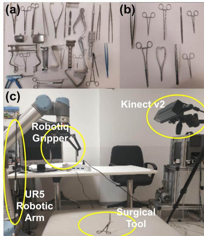
**Figure 3.** The experimental setup with surgical tools is presented. In (a), the different shapes of 27 surgical tools for training and testing (seen objects) are shown. In (b), the 9 new surgical tools for validation (unseen objects) are displayed, and in (c), the experimental setup is provided. The experimental setup is composed of a UR5 manipulator, a Robotiq gripper, a vision sensor, and a surgical tool.
