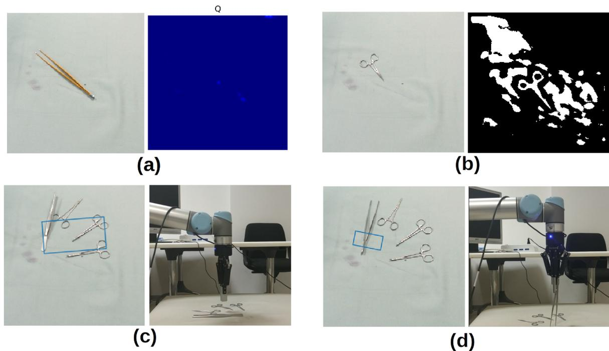
**Figure 7.** Failure examples: (a) no grasping box detection based on  $q$  value, (b) wrong segmentation as well as no grasping box detection, (c) wrong grasping box, and (d) tool falling in a cluttered environment.
