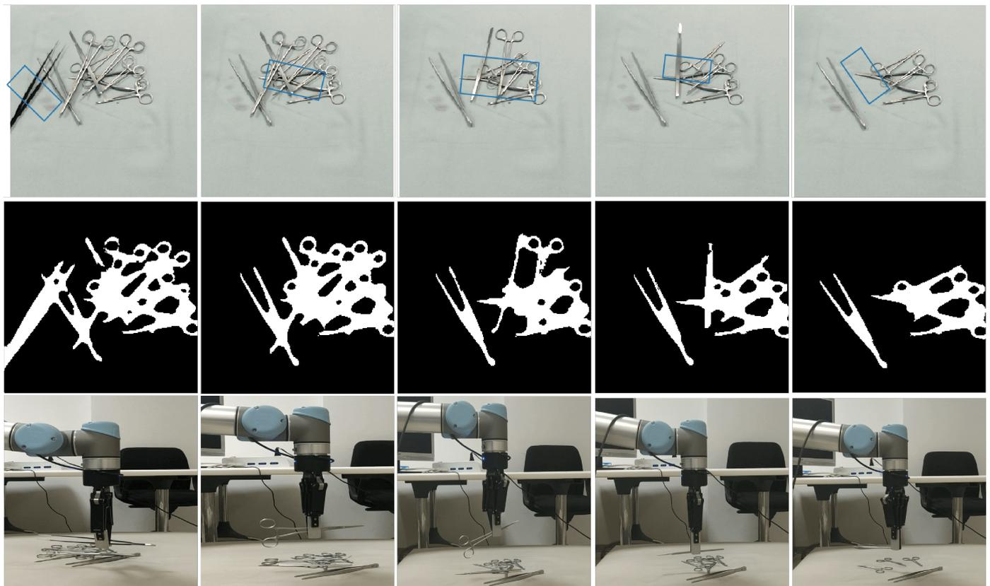
**Figure 6.** The process of grasping multiple surgical tools in a cluttered environment. During the grasping performance, GG-CNN2 searched a new grasping rectangle, and with color-based segmentation on the scene in the first and the second rows. In the last row, the robotic arm and gripper grasp the tools based on the networks' information.
