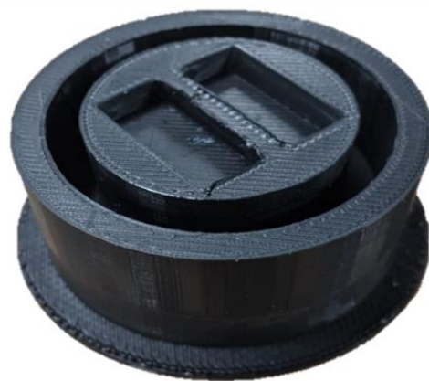
Figure 11. Three-dimensionally printed mold where liquid urethane is poured and cured.
