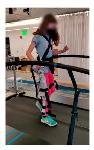
**Figure 4.** Pediatric participant walking on the instrumented treadmill while wearing the adjustable pediatric exoskeleton.
