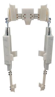
Figure 1. CSU Adjustable Pediatric Exoskeleton.
