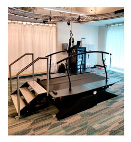
Figure 3. R-Mill instrumented treadmill.
