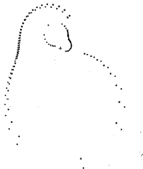
Figure 16. The three Burmester curves for a triad in six precision positions. There are two circle-point curves (corresponding to the two moving pivots) and one center-point curve [21] (p. 86).
