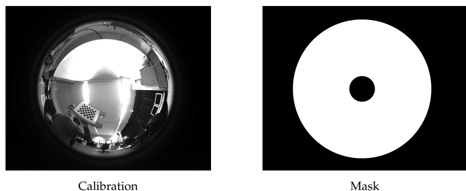
Figure 19. Camera calibration and mask image. The calibration image is one example of several images collected showing a checkerboard pattern [21]. These calibration images were used to obtain the camera parameters necessary for “unrolling” the image into a panoramic representation [20,22]. The mask image was used for exposure control and preprocessing to ignore those regions of the image which were not exposed at all or contain no meaningful information, such as the typically overly bright ceiling. The ring-shaped region extended from about 20^\circ on the inner side to about 110^\circ on the outer side, or in terms of elevation and depression, up to 70^\circ above and 20^\circ below the horizon.
