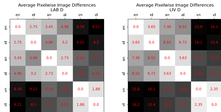
Figure 20. Plot of the average pixelwise image differences between all tilt-correction solutions. The LAB and LIV database are reported separately as the ranges of tilt and thus the expected deviations were different (LIV comprised more tilt). The results were averaged by taking the mean per method over all images contained in the database. For the tilt correction, the ground-truth tilt parameters as recorded in the database were used. The image difference measure is a symmetric distance measure, therefore the plotted matrices are symmetric about the main diagonal as well. With a stronger approximation, the effect of the different interpolation methods becomes smaller. The exact e^* and approximate solutions a^* are more similar to each other than to the vertical approximation v^* .
