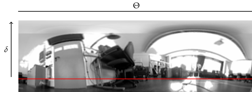
Figure 4. Angular coordinates of pixels in the panoramic image: modified spherical coordinates where the vertical angle \delta is measured from the horizon (red line) which lies somewhere inside the vertical range of the image. The horizontal angle \Theta runs from left to right in the reading direction.
