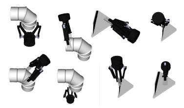
Figure 13. Some examples of generated grasping postures used in the current proposal.
