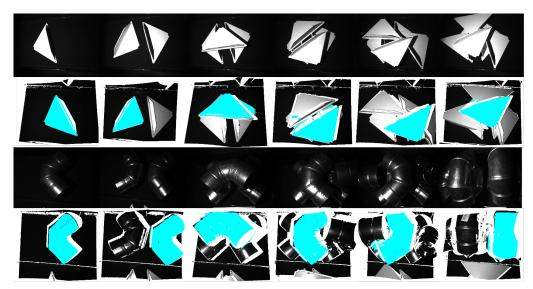
**Figure 18.** First scenario perception results. (**1st and 3rd row**) Original image; (**2nd and 4th row**) segmentation result.
