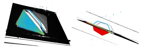
Figure 20. Proposed pipeline matching error. (Left) Point-cloud segmentation; (Right) Point-cloud matching
