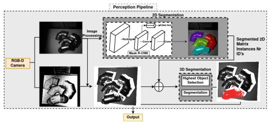
Figure 4. Perception pipeline for image segmentation (adapted from [30]).
