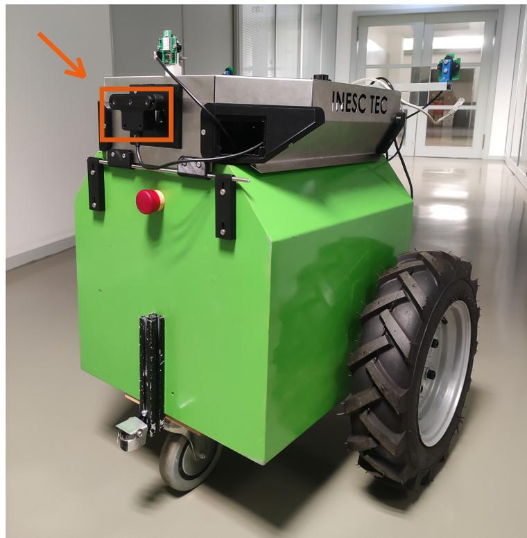
**Figure 3.** Robotic platform with OAK-D (surrounded by an orange rectangle).
