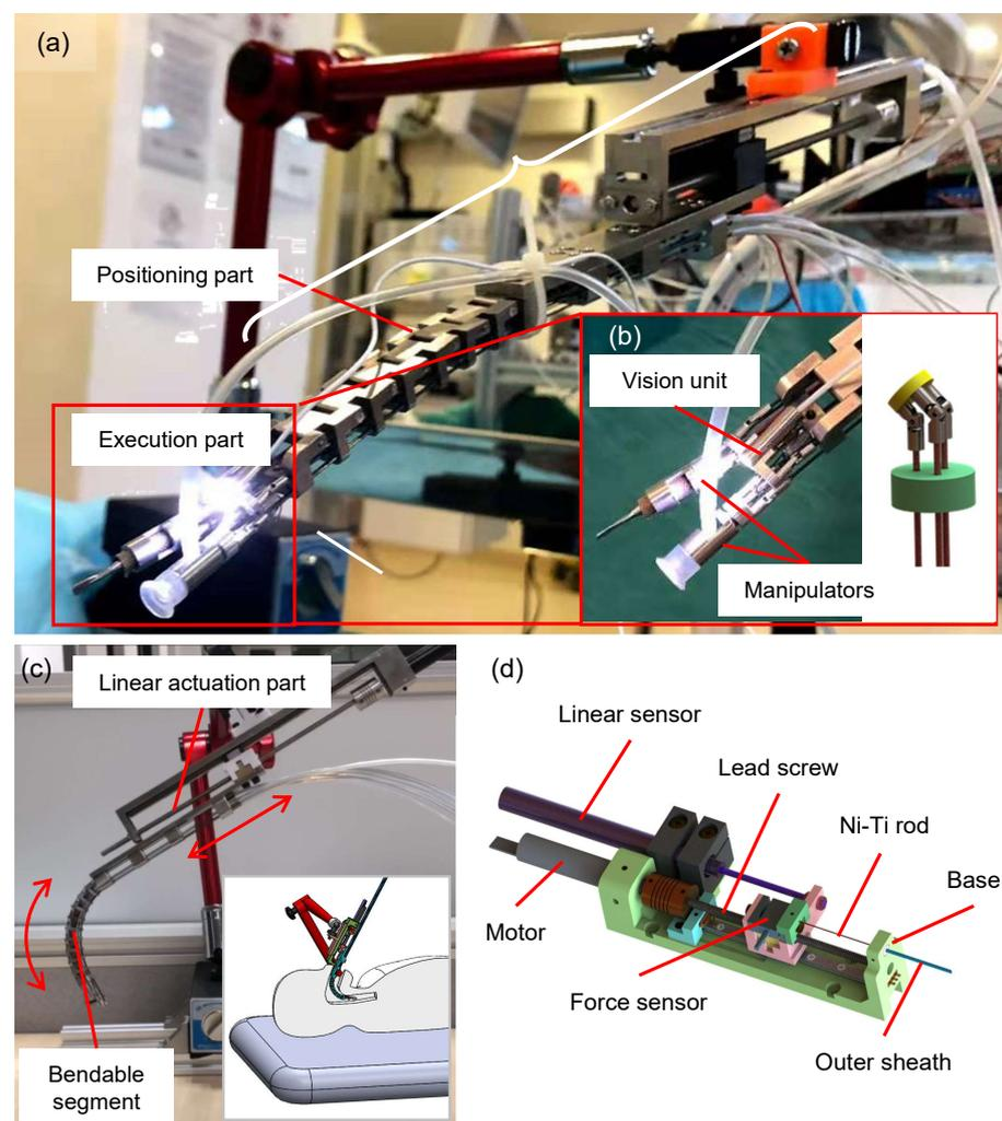
**Figure 1.** Overview of the surgical robot. (a) Prototype. (b) Execution part. (c) Positioning part. (d) Part of the actuator to drive one Ni-Ti rod.
