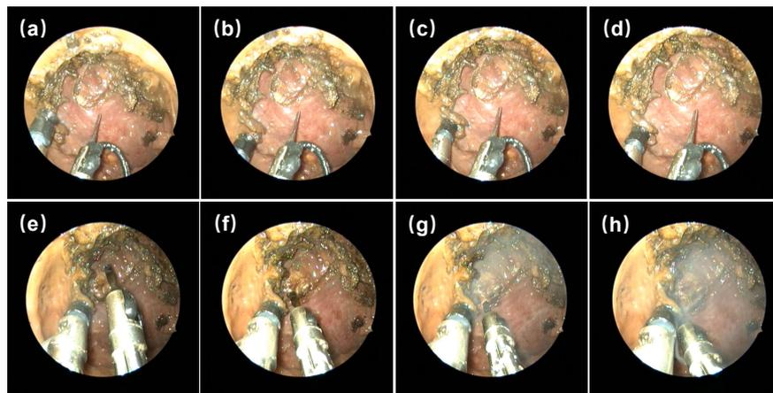
**Figure 4.** Endoscopic view of manipulators during the cadaver trial. (a–d) The left manipulator is equipped with vacuum suction to grasp the target tissue. (e–h) The process of the right manipulator equipped with the monopolar electrotome to cut the target tissue.
