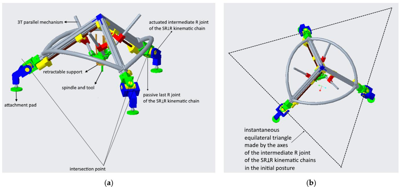
**Figure 8.** The addition of SRLR (SU) chains to the 3T mechanism by using the second U joint configuration in which (a) the last R joints of the SRLR kinematic chains intersect at a common point while the intermediate R joints are actuated and (b) the axes of the intermediate R joints of the SRLR kinematic chains make an instantaneous equilateral triangle in the initial posture.
