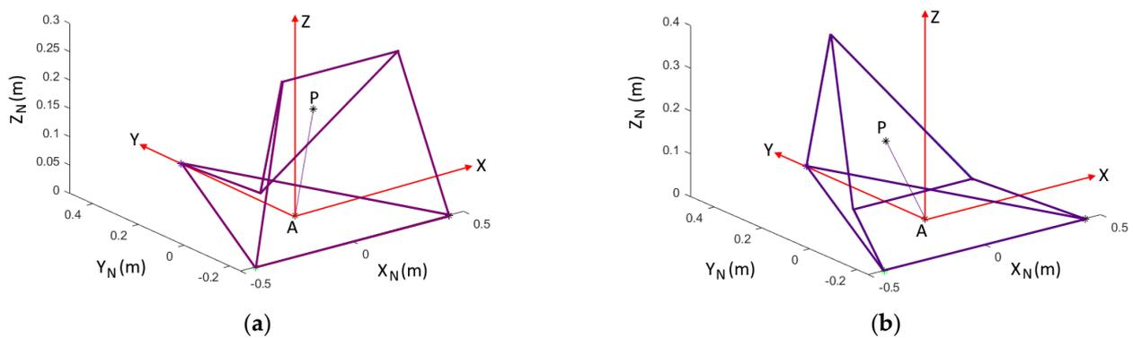
**Figure 24.** The optimized 3SU mechanism with the rotational range of the S and U joints between  $-80$  deg and  $80$  deg tilted at (a)  $\theta_x = -70$  deg,  $\theta_y = \theta_z = 0$  and (b)  $\theta_x = 60$  deg,  $\theta_y = \theta_z = 0$ .
