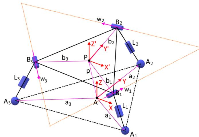
Figure 11. The schematic of the 3SPR mechanism.
