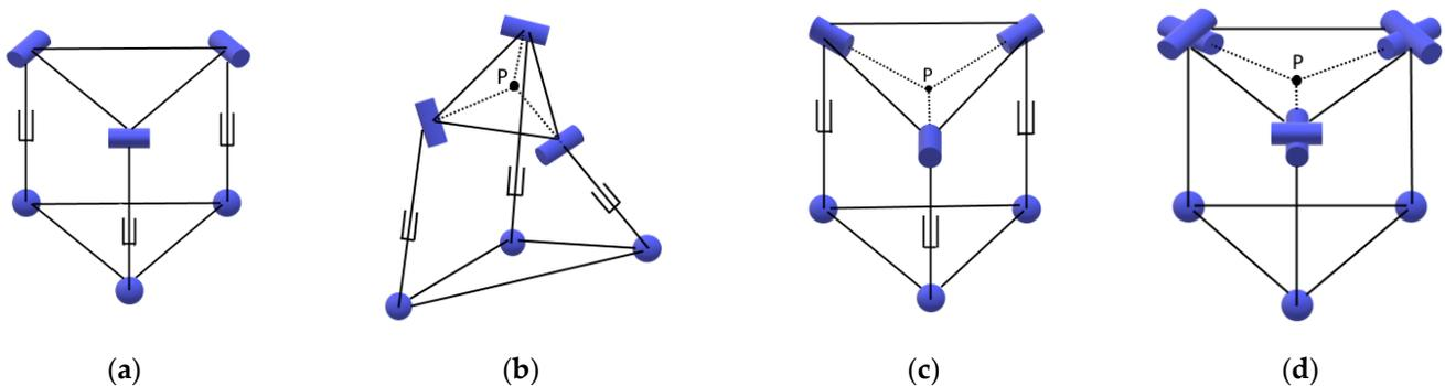
**Figure 16.** (a,b) Two configurations having architectural singularities in the 3SPR mechanism, (c) the constraint singularity configuration in the 3SPR mechanism, and (d) an architectural singularity in the 3SU mechanism.
