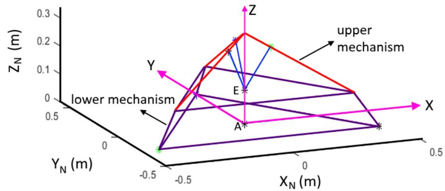
**Figure 14.** Three-dimensional view plot of the 3SPR-3PRPR mechanism with the end-effector E in an orientation of (0, 0, 0) and position coincident with the center of the moving platform of the lower mechanism.
