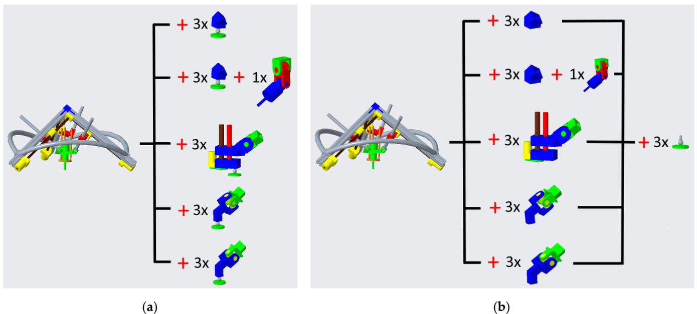
**Figure 19.** Two possible reconfiguration scenarios using modularity: (a) the attachment pad and spherical joint are included in each module, and (b) the attachment pad and spherical joint are made as separate modules.
