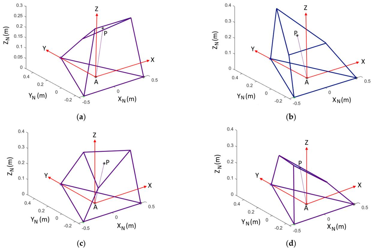
**Figure 26.** The optimized 3SU mechanism with the rotational range of the S and U joints between  $-30$  deg and  $30$  deg tilted at (a)  $\theta_x = -10$  deg,  $\theta_y = \theta_z = 0$ , (b)  $\theta_x = 10$  deg,  $\theta_y = \theta_z = 0$ , (c)  $\theta_x = 0$ ,  $\theta_y = -10$  deg,  $\theta_z = 0$ , and (d)  $\theta_x = 0$ ,  $\theta_y = 10$  deg,  $\theta_z = 0$ .
