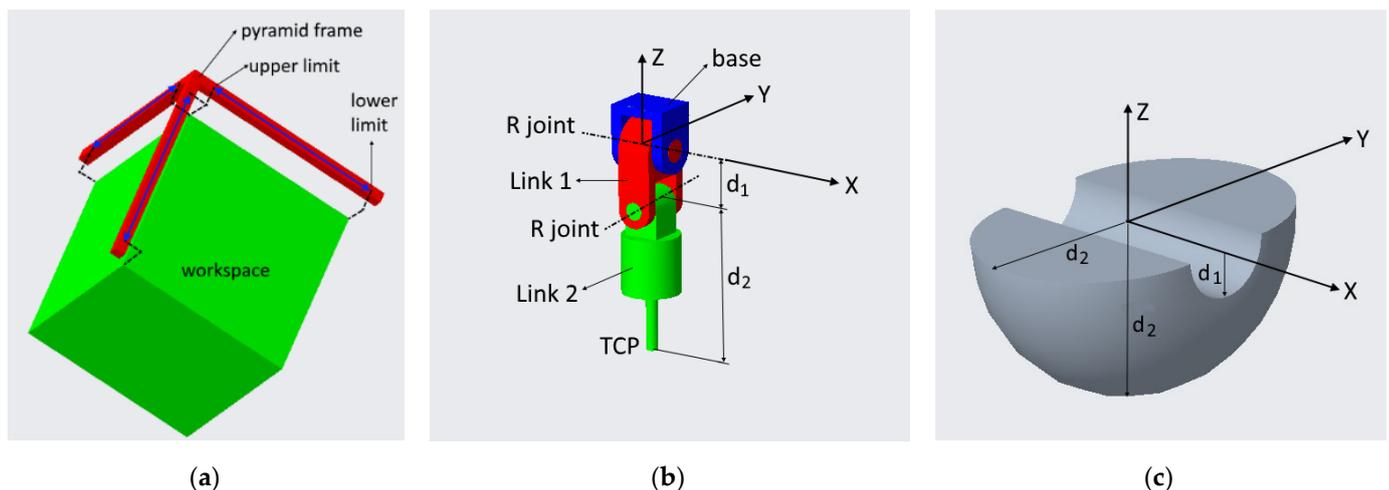
**Figure 17.** (a) The workspace of the 3T mechanism, (b) serial RR mechanism with two non-zero links, and (c) total orientation workspace of the serial RR mechanism shown in (b) given the tilting range of both the R joints between  $-90$  and  $90$  degrees.
