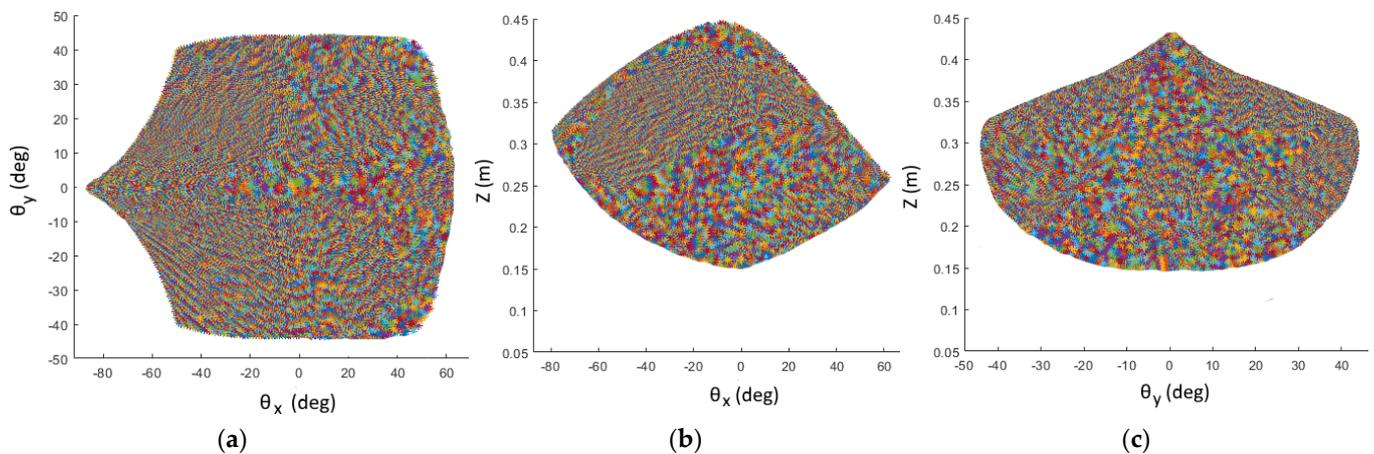
**Figure 23.** (a–c) Two-dimensional plots of the orientation workspace of the optimized 3SU mechanism with the rotational range of the S and U joints between  $-80$  deg and  $80$  deg. The dots, regardless of their color, represent the reachable tilting angles.
