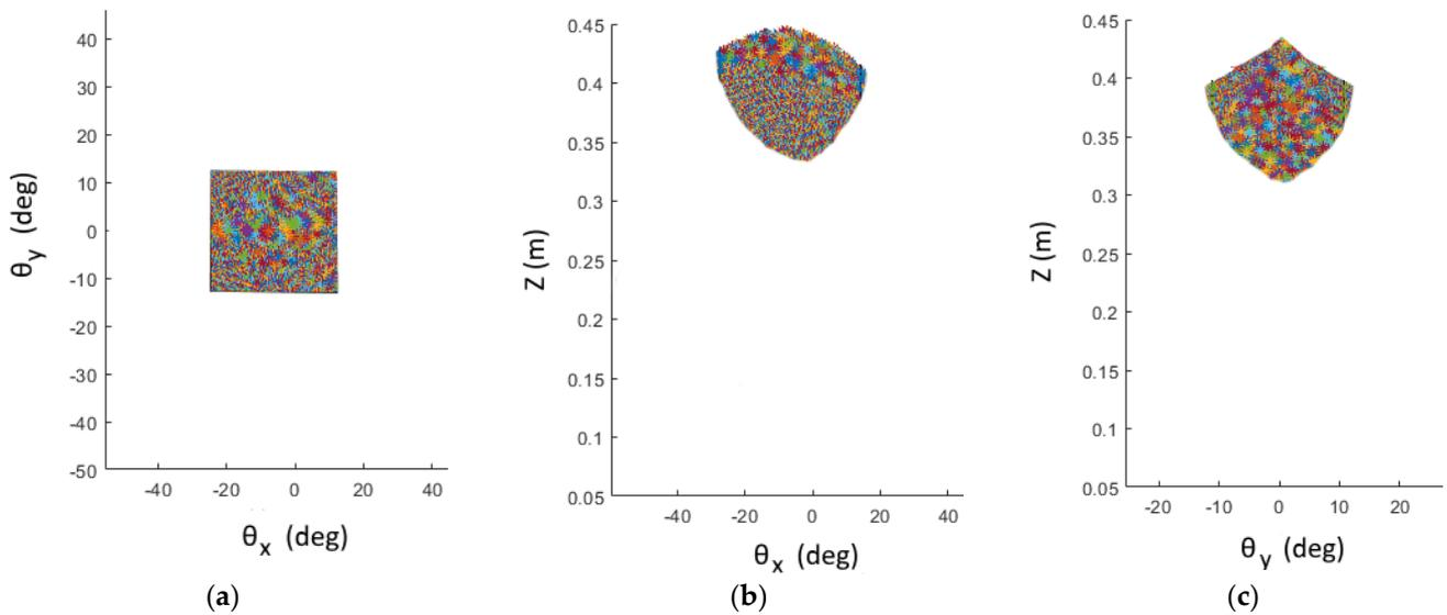
**Figure 25.** (a–c) Two-dimensional plots of the orientation workspace of the optimized 3SU mechanism with the rotational range of the S and U joints between  $-30$  deg and  $30$  deg. The dots, regardless of their color, represent the reachable tilting angles.
