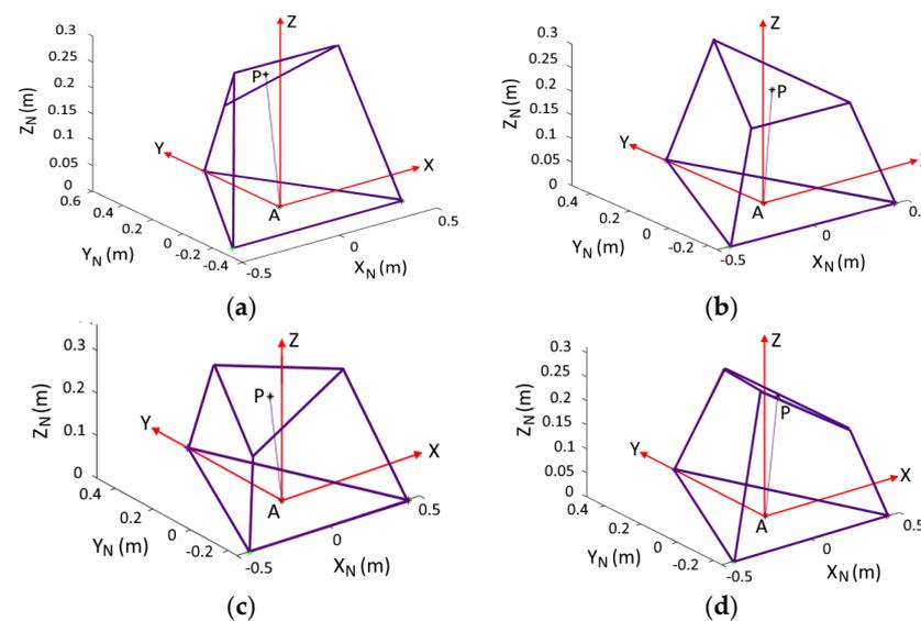
**Figure 22.** The optimized 3SPR mechanism tilted at (a)  $\theta_x = -20 \text{ deg}$ ,  $\theta_y = \theta_z = 0$ , (b)  $\theta_x = 10 \text{ deg}$ ,  $\theta_y = \theta_z = 0$ , (c)  $\theta_x = 0$ ,  $\theta_y = -15 \text{ deg}$ ,  $\theta_z = 0$ , and (d)  $\theta_x = 0$ ,  $\theta_y = 15 \text{ deg}$ ,  $\theta_z = 0$ .
