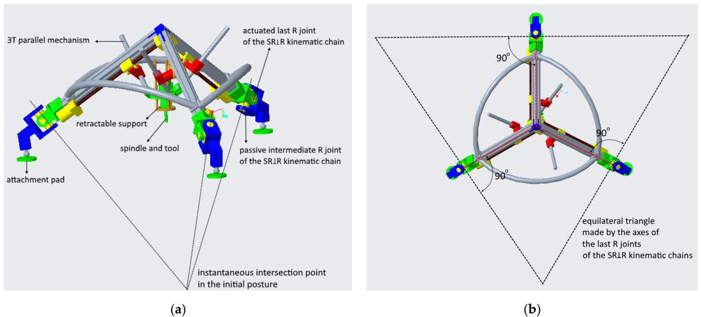
**Figure 7.** The addition of SRLR (SU) chains to the 3T mechanism by using the first U joint configuration in which (a) the intermediate R joints of the SRLR kinematic chains intersect at a common point in their initial posture while the last R joints are actuated and (b) the axes of the last R joints of the SRLR kinematic chains are fixed in a perpendicular position with respect to the segments of the pyramid frame, making an equilateral triangle.
