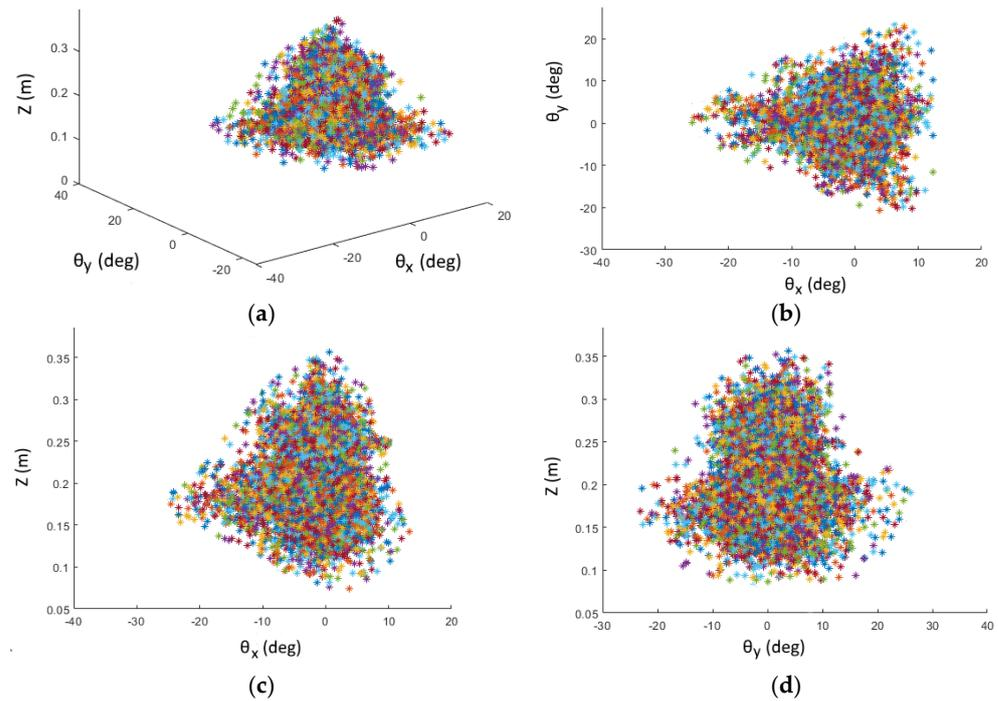
**Figure 21.** (a) Three-dimensional and (b–d) two-dimensional plots of the orientation workspace of the optimized 3SPR mechanism. The dots, regardless of their color, represent the reachable tilting angles.
