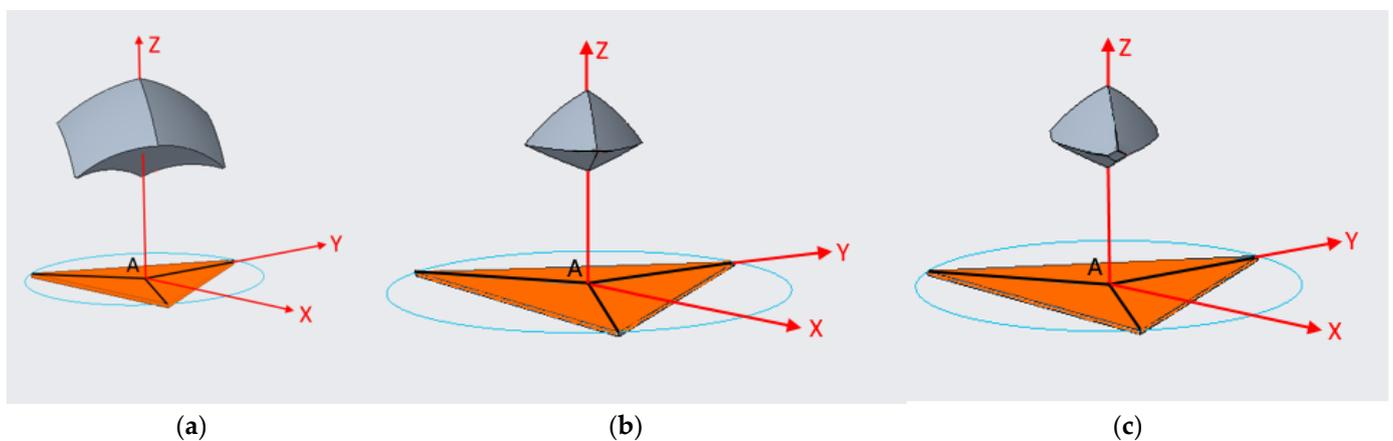
**Figure 18.** The total orientation workspaces of the 3SPR mechanism with (a)  $R = 0.3$  m,  $L_{i, \min} = 0.2$  m,  $L_{i, \max} = 0.6$  m, and (b)  $R = 0.5$  m,  $L_{i, \min} = 0.2$  m,  $L_{i, \max} = 0.6$  m, and (c) the total orientation workspace of the 3SU mechanism with  $R = 0.5$  m,  $r = 0.3$  m. All the mechanisms use the S joints with a rotational motion range between  $-30$  and  $30$  degrees.
