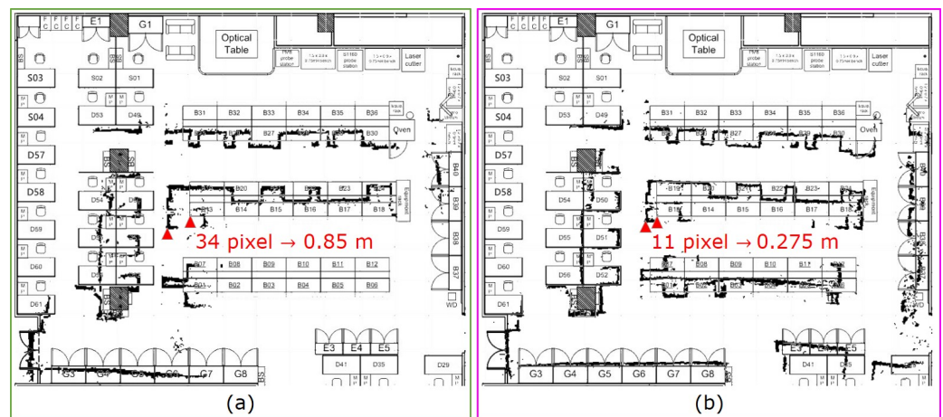
Figure 10. Map alignment result of the building blueprint and sensor map: (a) based on two key points; (b) based on three key points.
