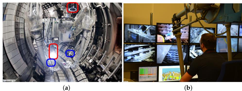
**Figure 2.** JET's remote handling system: (a) MASCOT manipulator (robotic system) inside the JET vacuum vessel; and (b) operator, interface and viewing system. Red and blue squares represent the HD and ancillary cameras, respectively, mounted on MASCOT.
