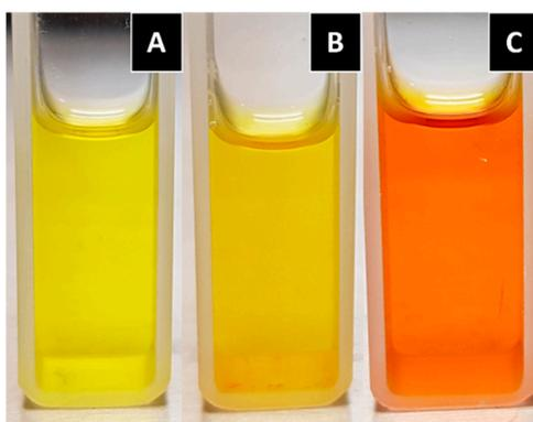
**Figure 3.** Curcumin dissolved in different mediums. (A) Curcumin in an acidic solution (pH 3.5); and (B) curcumin in a neutral solution (pH 7.4); both with the addition of 1% Tween 80 in order to increase solubility. (C) Curcumin in a basic solution (pH 12).
