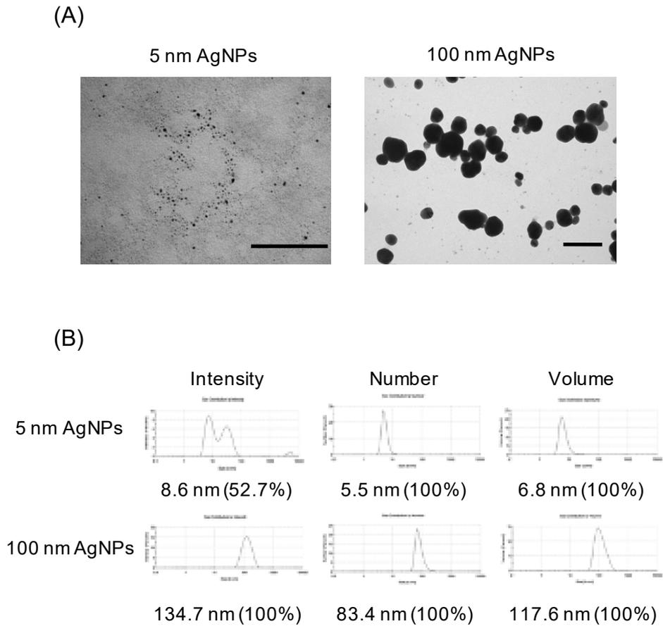
**Figure S1. Characteristics of AgNPs.** (A) TEM images of AgNPs show that 5 nm and 100 nm nanoparticles are relatively uniform in size and well distributed. Scale bar: 200 nm. (B) DLS analysis by number reveals mean sizes are 5.5 nm for 5 nm AgNPs and 83.4 nm for 100 nm AgNPs. For DLS analysis, AgNPs were dispersed in RPMI 1640 containing 1% FBS.
