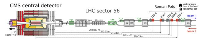
**Figure 3.** Schematic layout of the CMS Proton Precision Spectrometer (PPS) located in LHC sector 56. The accelerator magnets are displayed in gray, while the collimator system parts are highlighted in green. The detector units, marked in red, are those used by PPS during Run 2. The figure is taken from Ref. [28].
