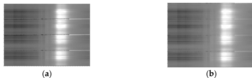
Figure 2. Normalized noise reduction results of channels: (a) before normalization of channels, (b) after normalization of channels.
